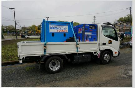
At the compact size that I can put on a 2t vehicle, it is projection speed of the world fastest water jet blast. As for 2L (in 200Mpa), quantity of water to use for one minute is the littlest in the world.
